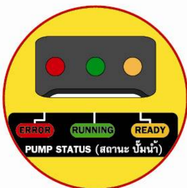
LED Status (On terminal box)
